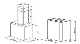
**Titan** is a modern and stylish cooker hood offering many options. It is available in standard widths of 60 or 90 cm, with or without chimney. Titan is also available in custom heights and widths, and in all our metals and colours.
